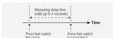
\* If the pedal is not pressed twice within 4 seconds, the setting for the tap function is not valid, and the delay time for the patch will not change.
