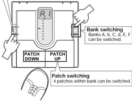
Bank/patch switching when Bank Hold is on
