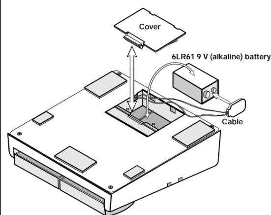
1. Turn the 508 upside down and open the cover of the battery compartment. (Push the catch to unlock the cover, then lift it up.)
